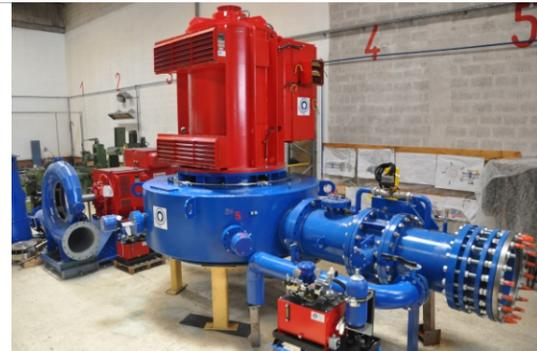
Quality starts already with the design. Siapro design both vertical and horizontal axis Pelton turbines with up to 10 MW.
