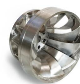
We design and supply high quality casted runners for Francis turbines made of 1.4317 material. Runners are finally machined, polished and balanced.
